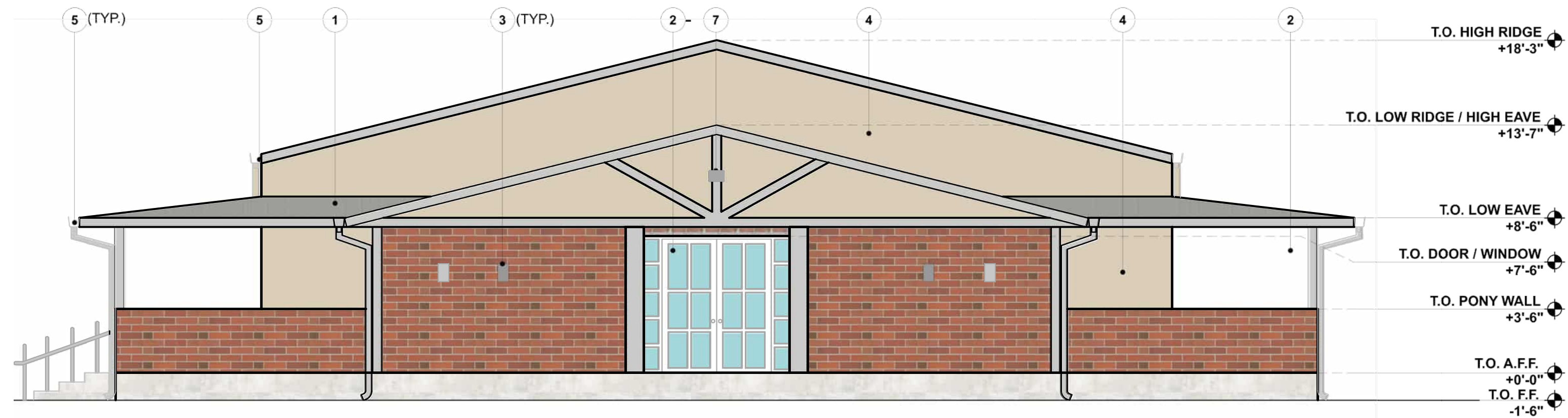
1 WEST (FRONT) ELEVATION @ ASSEMBLY HALL SCALE: 3/16" = 1'-0"
